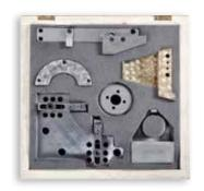
The **equipment kits,** are realised according to the **SMED** analysis to reduce the set up time.
